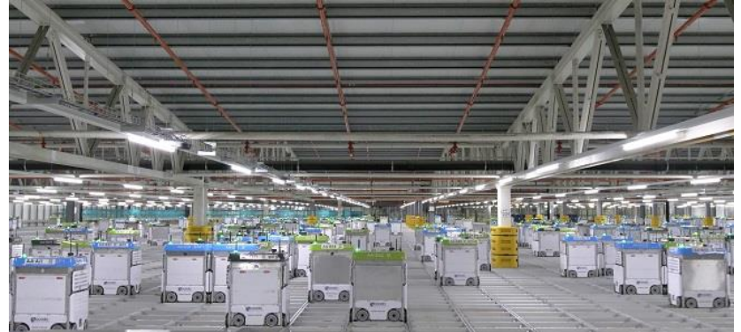
An Ocado automated distribution centre utilising their smart automated packing systems.
